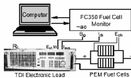
**Figure 1.** Two Ballard Nexa™ PEFC stacks connected in parallel operation for ac impedance measurement.
