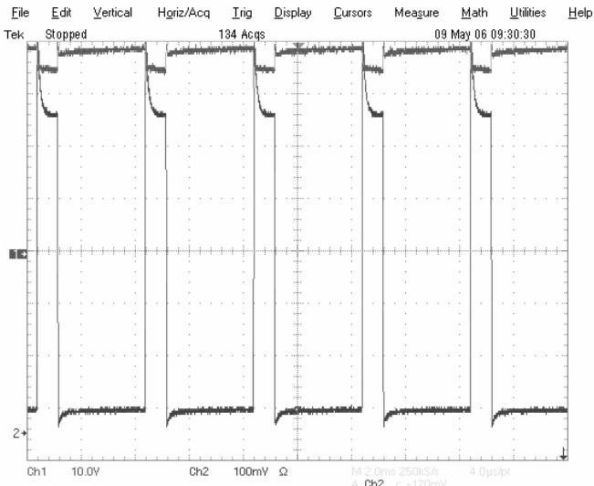
**Figure 3.** Two Nexa<sup>TM</sup> stacks (#881 and #515) operated in parallel and pulse tested at a total current (bottom line) of 60 A and pulse voltage (top line) between 35.4 V and 39.4 V at 250 Hz frequency and 20% duty cycle. Before tests at 60 A, Nexa<sup>TM</sup> stack #881: Ts=54.5°C, Es=31.36 V, Is=29.45 A, Ps=925 W; Stack #515: Ts=60.6°C, Es=31.66 V, Is=36.47 A, Ps=1155 W.
