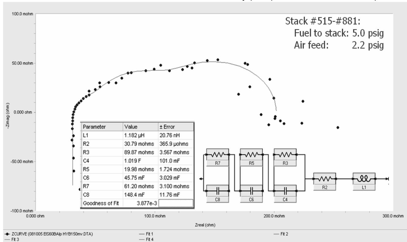
**Figure 2.** Nyquist plot, equivalent circuit diagram, and simulated physical elements of two Ballard Nexa™ stacks in parallel operation using a LR(RC)(RC)(RC) circuit fit at a load of 60 A.
