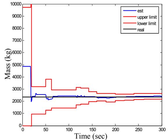
**Figure 6: Mass Estimation Results, Chrysler Proving Grounds**
