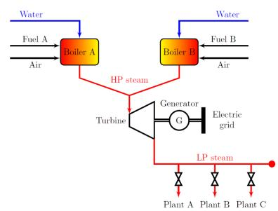
Figure 1 shows a simplified flowsheet of the system. Here, two boilers generate high pressure steam by burning different fuels, Fuel A and Fuel B respectively. The high pressure (HP) steam is expanded to low pressure (LP) in a turbine which drives a generator to produce electric power to the grid. The low pressure steam is distributed through a steam network to each consumer (Plant A, B,C).
