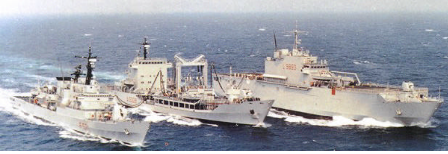
Figure 6.8: Italian supply ship “Vesuvio” refueling two ships at sea. Courtesy: Hepburn Engineering Inc.
