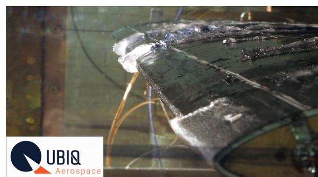
Figure 5: Anti-icing system in operation with partially unheated zones. Photo: R. Hann
