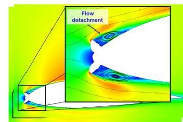
Figure 4: CFD results for icing
