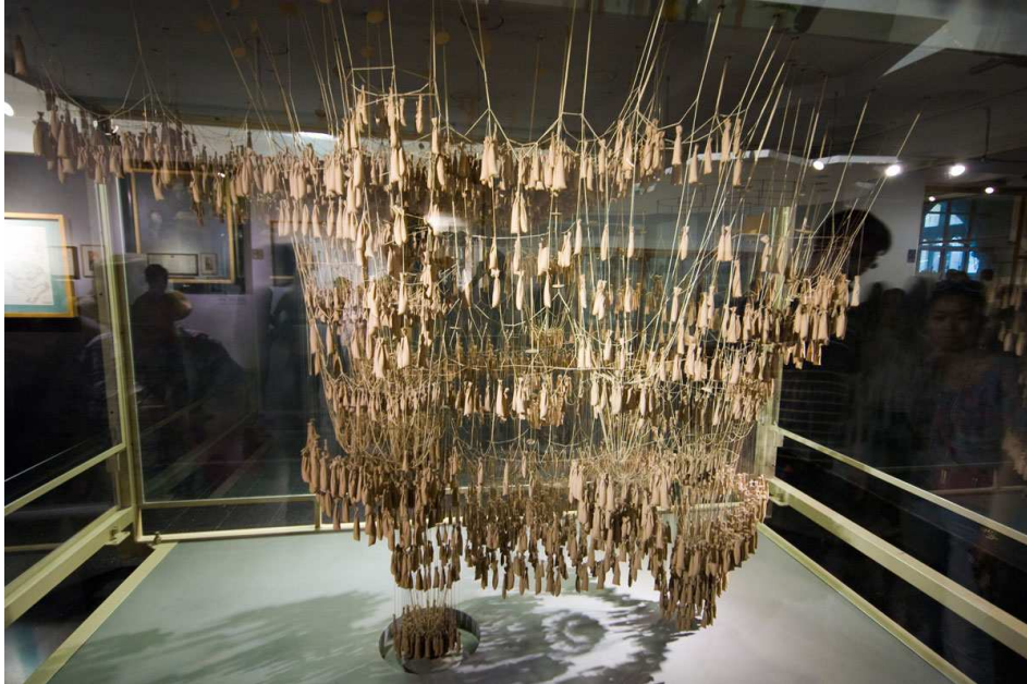
Figure 1.4: Gaudi: funicular model of Sagrada Familia: A method that Gaudi used to design buildings based on catenary arches (the arches that result from hanging chains – the same method used in many medieval cathedrals) – Gaudi used string and little sand-filled bags to load the strings. The result is a geometrical model that represents the structural elements upside down. This is a reconstruction, which is based on a photographs of the original. The original was lost when Gaudi’s studio burned down. It is displayed in the ‘museum’ at Sagrada Familia. One of the most fascinating exhibition pieces.
