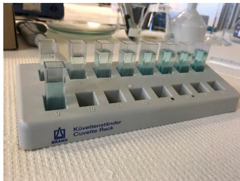
Figure 5: Cuvettes for measurement of absorbance with the UV-Vis Spectrophotometer
