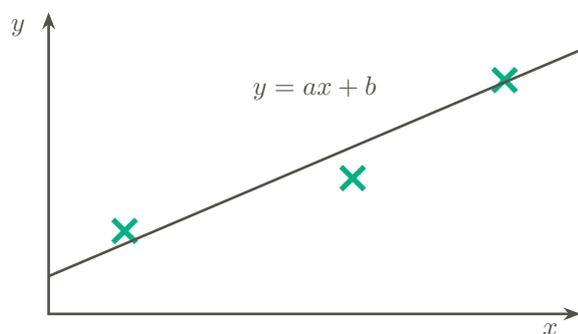
Figure 3: Example of a linear calibration curve. The  $x$  is the bit reading measured, which has to be expressed as a percentage,  $y$ , using regression.
