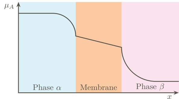
Figure 1: Illustration of chemical potential profile across the membrane and the two phases.
