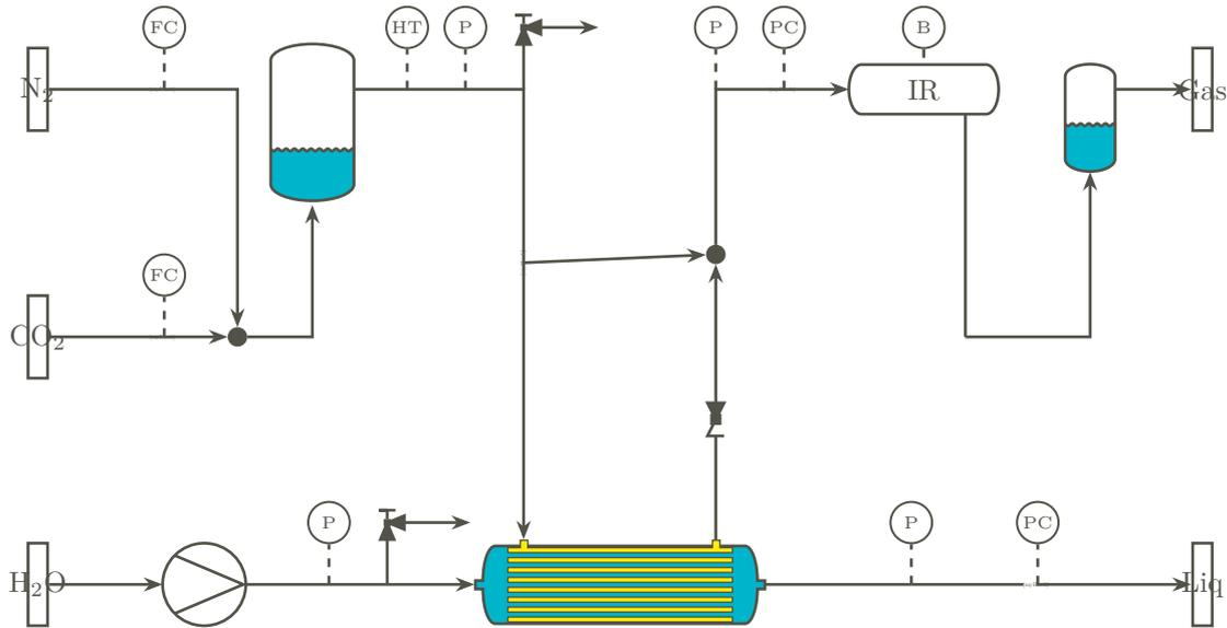
Figure 2: This figure illustrates the experimental setup for the membrane contactor rig. The units are explained in table 1.
