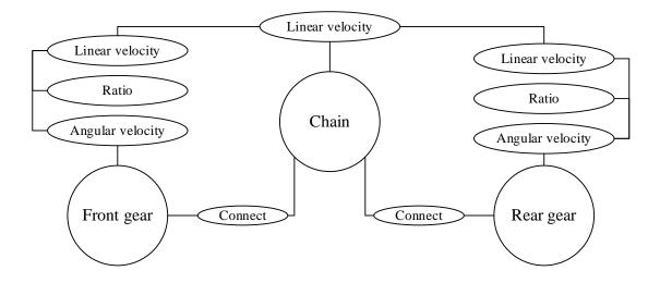
Figure 7. Bicycle transmission metamodel.
