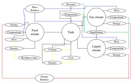
Figure 9. Metamodel for an adiabatic flash tank.
