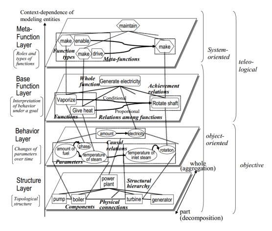
Figure 4. Hierarchy of a target object (power plant).
