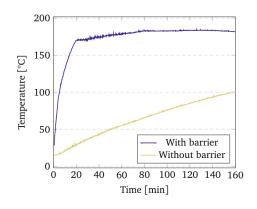
Test heating with and without barrier
