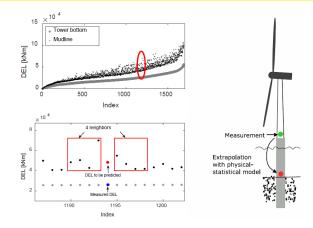
How to extrapolate fatigue damage from measurements at a different location?)
