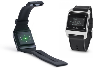
Fig. 2. The back side ( left ) and the front side ( right ) of Basis B1.
