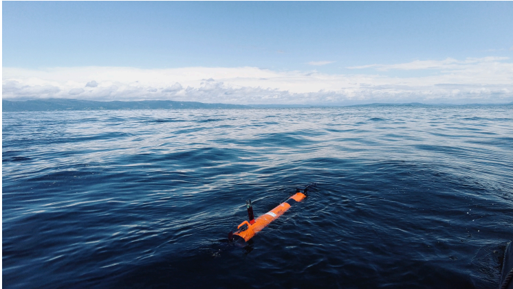
Fig. 9: LAUV Roald is on expedition with an adaptive sampling algorithm onboard. The AUV is about 2 m long and runs at about 1 m/s. It is doing a 3D sampling mission at depths ranging from 0.5 to 5.5 m.
