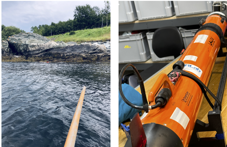
Figure 4.3: The field experiment yielded some unexpected results, as evidenced by the image on the left which shows an AUV stranded close to the shore. The image on the right displays an AUV with its wings damaged.
