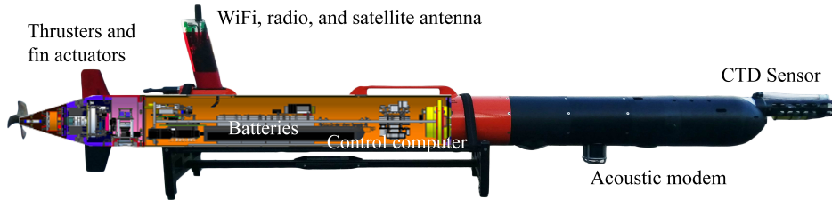
FIG 9. The commercially available Light Autonomous Underwater Vehicle (LAUV) platform for upper water-column exploration used in our experiments.
