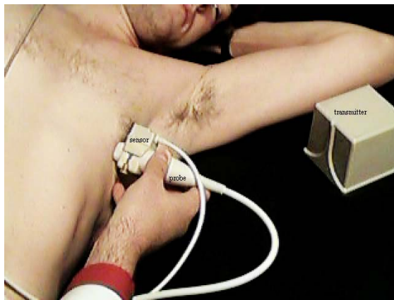
Figure 1 The photo shows the ultrasound probe with the magnetic position locating device. The sensor is mounted on the probe while the transmitter is placed 25-60 cm from the sensor.
