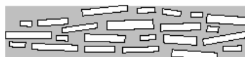
Fig. 1. Vertical cut of a dry-pressed clay sample; the platelet-shaped particles have a strong tendency to be aligned with the horizontal direction (the stress was applied vertically at dehydration).
