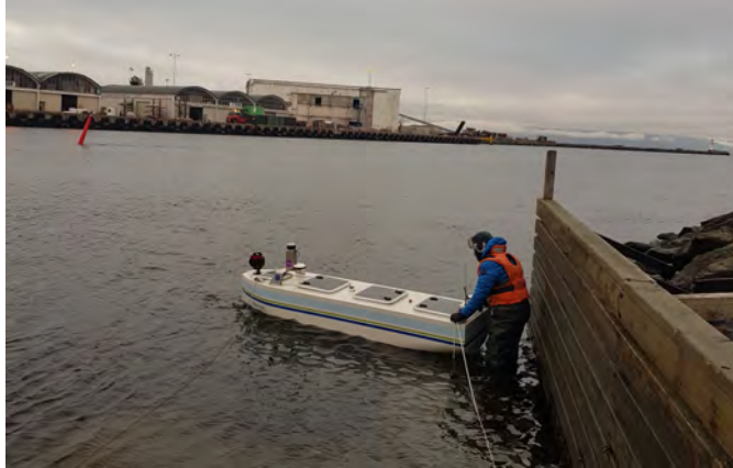
Figure 4.6: Testing synchronization setup. ReVolt was shaken and stirred to provide kinematic-data from the IMU
