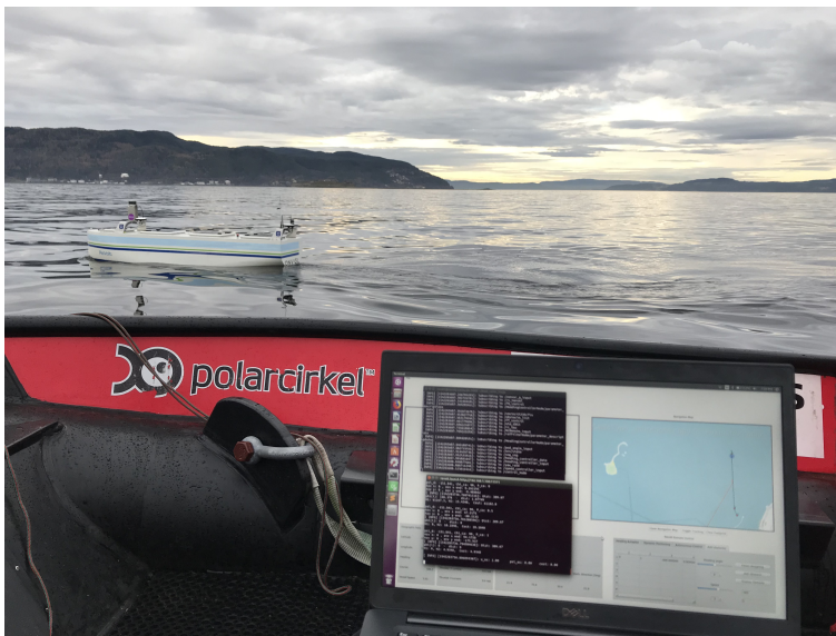
Figure 6.5: Mid-testing, where ReVolt is running a COLAV scenarios carefully monitored in the remote control station.
