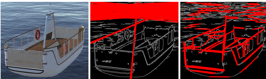
Figure 5.2: Original image, standard Hough line transform with no threshold, probabilistic Hough line transform.
