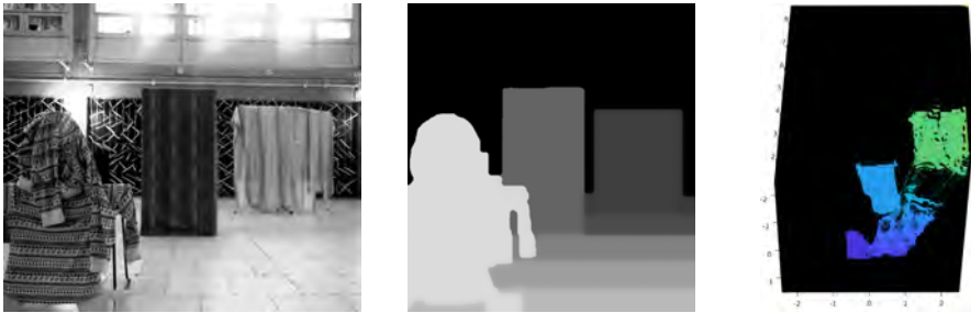
Figure 2.9: Example of scene with corresponding grey-scale disparity map and Point cloud
