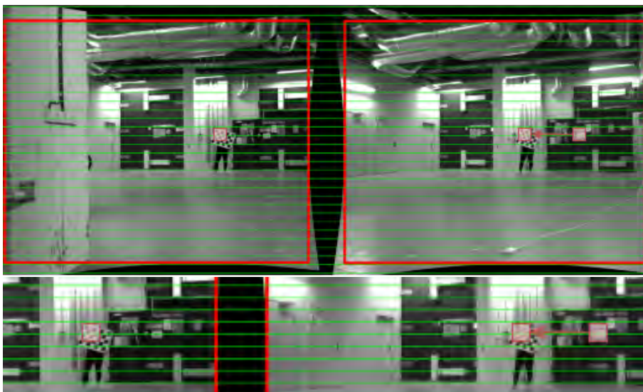
Figure 3.2: Block matching between two rectified images. The reference block in the left image is matched with different blocks on the same horizontal line in the right image.
