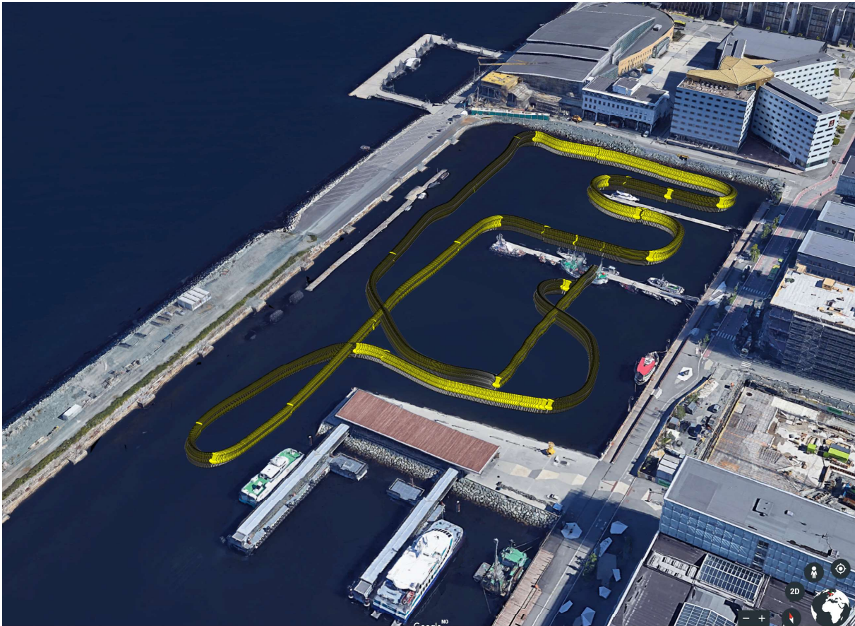
Figure 4.5: Screen-shot of the ferry's trajectory from which the data is logged. The almost straight line from the middle floating dock is the return, while the curved one is from shipping out. Longitude and Latitude was from a rosbag in MATLAB, converted to a .KML-file and uploaded in GOOGLE earth. Note that at the of the logging procedure, the boat count was higher, and the construction site on the right had become structure much visible to the LIDAR.
