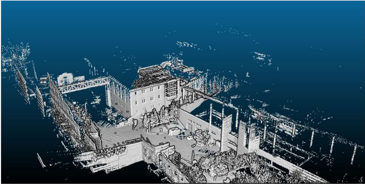
Figure 3.4: Example of map built by LOAM. Courtesy of [59].
