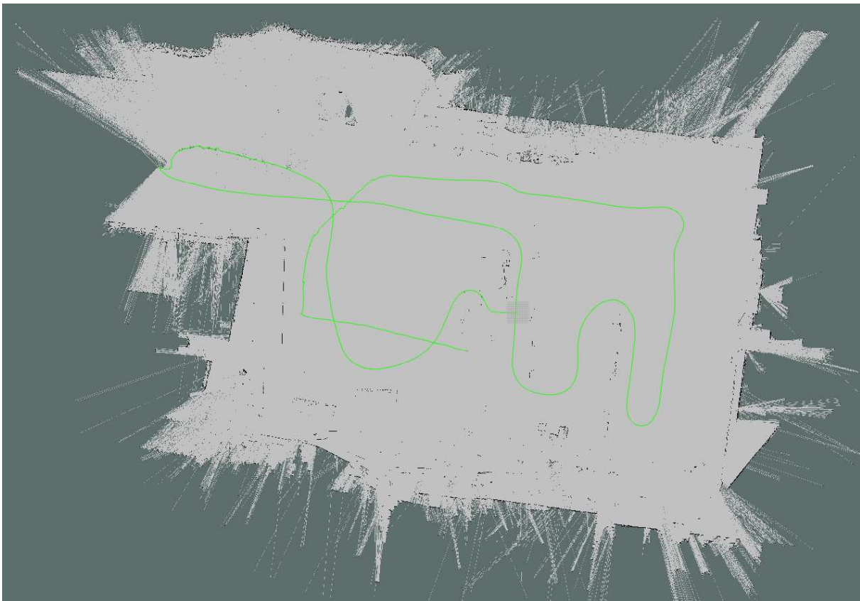
Figure 6.3: Resulting map and trajectory from running Hector-SLAM on the full data-set. Scans were filtered through the laser filter beforehand to get rid of rays hitting MilliAmpere.
