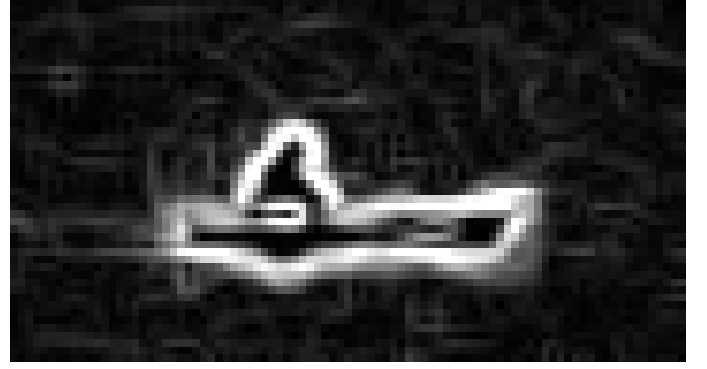
Fig. 3. Sobel gradient image of a detected boat
