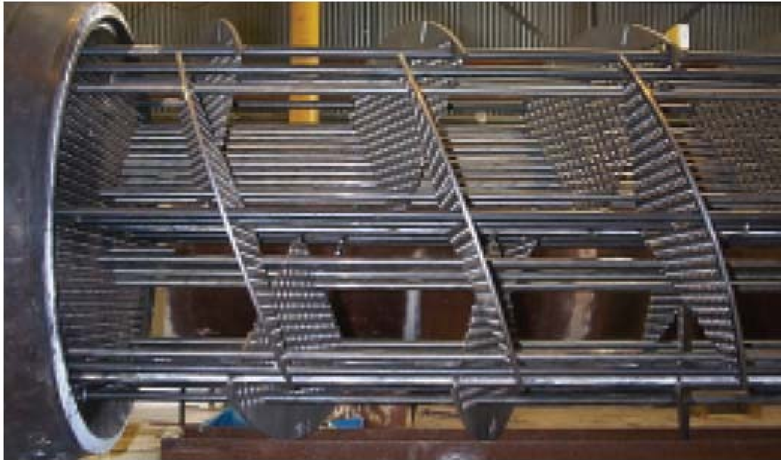
HELIFIN Heat Exchanger Tube Bundle in Fabrication
