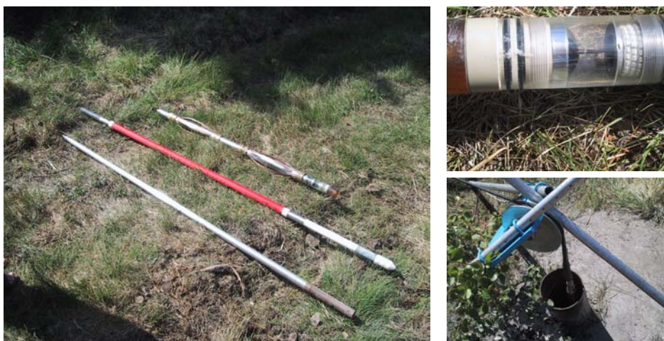
Figure 2: Left: Picture of the three probes. Upper right: detail of optical televiewer with hyperboloidal mirror, lower right: a probe is lowered into the borehole.
