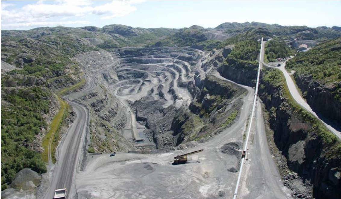
Figure 2. Tellnes open pit mine seen from West. Hanging wall (SW) to the right, footwall (NE) to the left. The top of the footwall is here at level ~250 m and the bottom is at level ~80 m.
