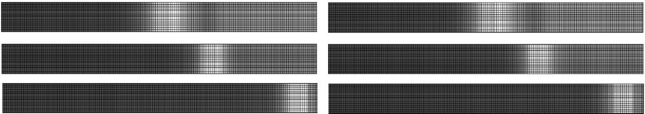
Figure 7: Density contours at  $t = 1000\Delta t_{ref}$ ,  $t = 5000\Delta t_{ref}$  and  $t = 10000\Delta t_{ref}$ . The reference explicit calculation is shown on the left and an implicit-explicit solution on the right. Inviscid terms are treated explicitly while viscous terms and chemistry are treated implicitly.
