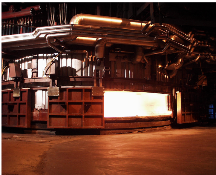
Figure 2.4: The top of a silicon furnace (Elkem 2004b).
