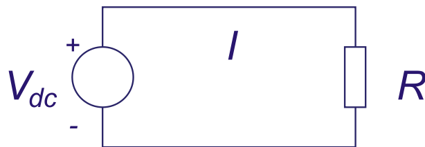
Figure C.1: Electrical circuit, with voltage source V_{dc} and a resistive load R .
