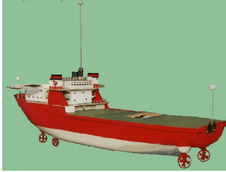
Figure 7.7: CyberShip I: Model ship scale 1:70.
